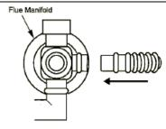
3. Fit the pipe stopper over the connection between the flue elbow and the manifold. Engage the hook and rotate it until it snaps against the body of the clamp.
