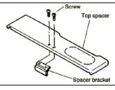
6. Install the wall bracket with two screws. Install the top spacer by clipping the spacer into the wall brackets and attaching it to the heater with 2 screws.
