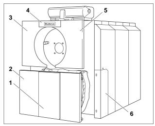
Fig. 28 Remove the front wall
