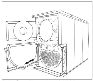
Fig. 30 Cleaning the secondary and third firetubes
