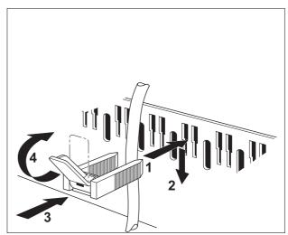
Fig. 18 Installation of the cable clips
