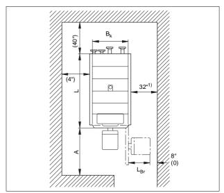
Fig. 2 Clearance dimensions for SB735 boilers
