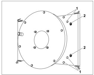
Fig. 6 Screws for opening the burner door
