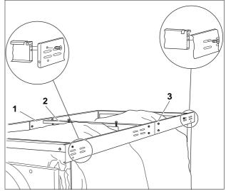
Fig. 12 Secure the longitudinal bracket with bolts suppplied
