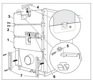
Fig. 26 installation of the rear wall section
