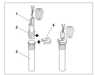
Fig. 20 Capillary tubes with sensor and sensor well
