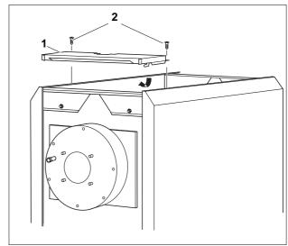
Fig. 16 Install the boiler front cover
