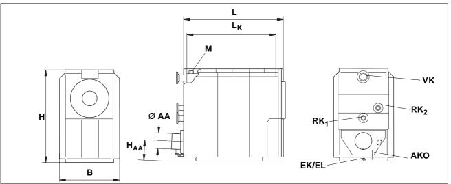
Fig. 1 Technical Data, Dimensions and Water Connections
