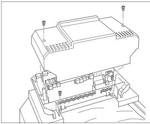
Fig. 17 Install the control panel
