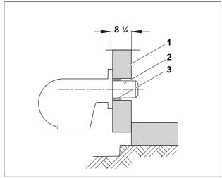
Fig. 22 Burner installation
